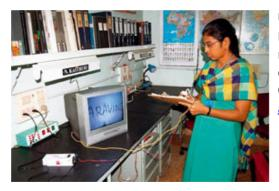
Using locally available CCTV cameras, the Instruments Maintenance Department at Aarvind – Madurai has come up with an innovative magnification system that can be connected to a local television. The details of this innovation has been published in the Journal of Community Eye Health, Volume 25; No:77. Click here to see the full article
