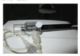
Instruments Maintenance team at Aravind – Salem developed an immersion prager shell – probe holding screw. While the supplier charges Rs. 788 for this small spare part, the cost of the product developed indigenously is just Rs. 30. This locally manufactured screw is also found to be exactly similar to the original one manufactured by the company.
