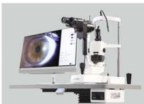
Hawk-i slit lamp attached with Third-i camera
