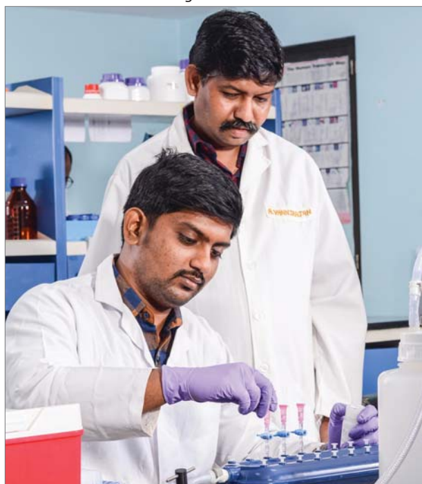
Nucleic acid extraction using Vacuum manifold
