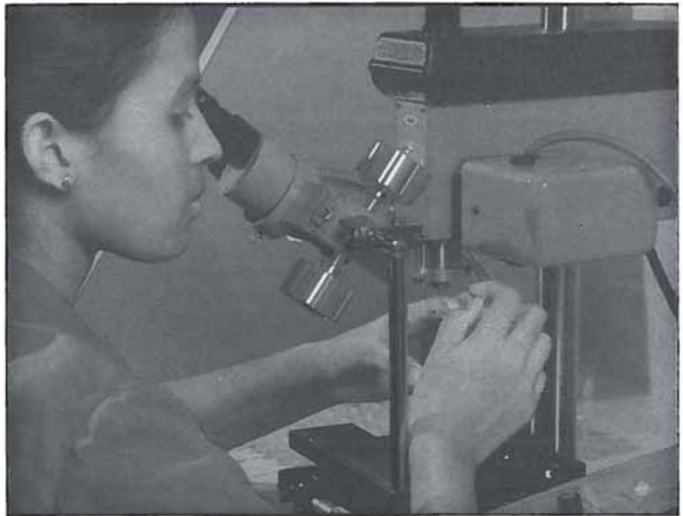
Drilling dialling holes
