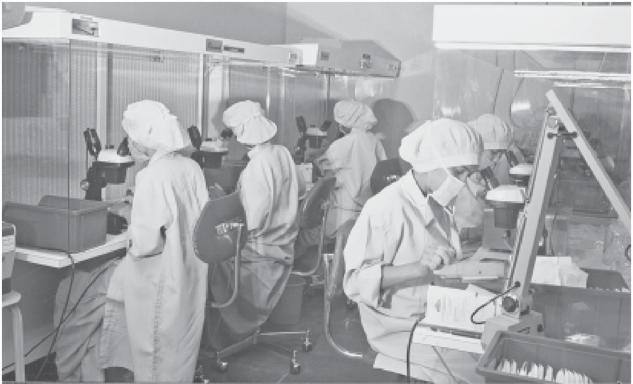
quality control and packaging of intraocular lenses in a clean room
