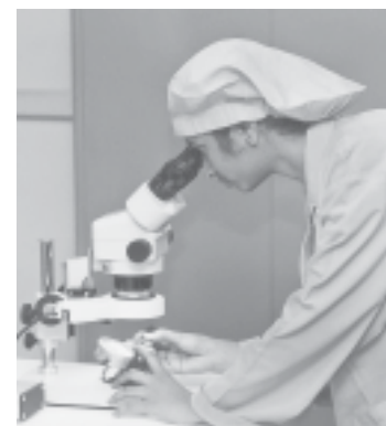
inspection of suture needles using precision measuring instrument
