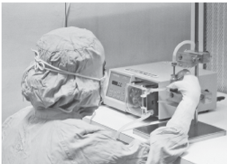
filling of ophthalmic drugs using a peristaltic pump
