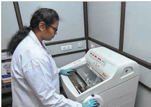
Frozen tissue sectioning using the Leica Cryostat
